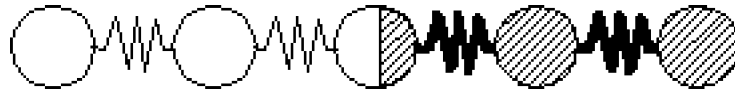
Fig. 4. A medium with two distinct materials, each with a different mass and elasticity.
