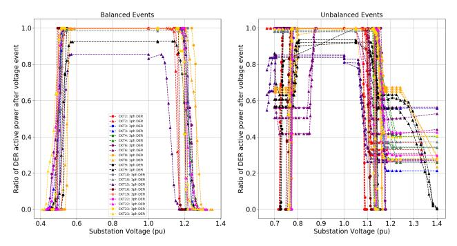
Fig. 9. Trip profile of distributed energy resources across multiple feeders with 100% distributed energy resource penetration with respect to load[108].
