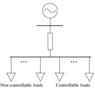
Fig. 17. Two-bus system used in simulations. Two groups of devices, non-controllable and controllable devices, are connected to the second bus, which is connected to a swing bus via a transmission line.
