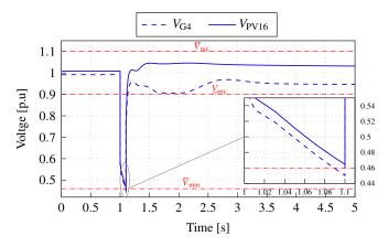
Fig. 7. Voltage at two different DER terminals compared to VRT requirements
