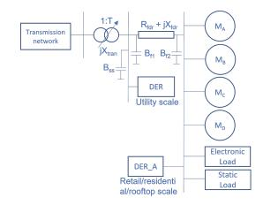
Fig. 8. Composite load model structure with equivalent motor load and distributed energy resource representation.
