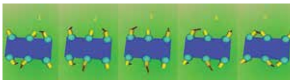
Figure 8. Simulation of the hexapod's walking sequence.
