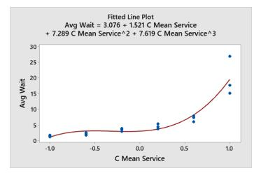
Figure 6: A cubic regression metamodel is not monotonic.
