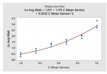
Figure 7: Transforming to ln(Avg Wait) reduces heteroscedasticity and improves fit.
