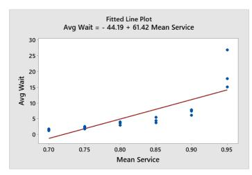
Figure 2: A regression metamodel fitted to the data, with intercept and linear term only.
