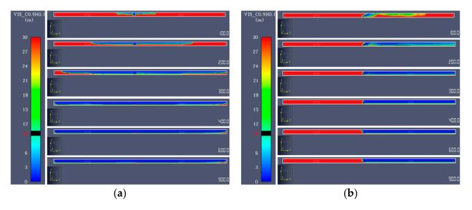
Figure 10. Changes in the longitudinal center section of visibility: (a) 0.5 m/s; (b) 3.6 m/s.
