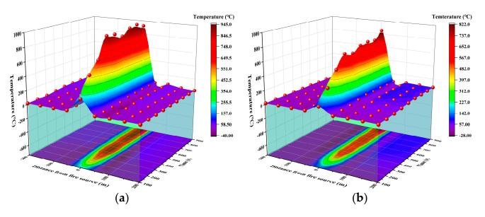
temperature difference between upstream and downstream was much larger than that at low ventilation velocity.
