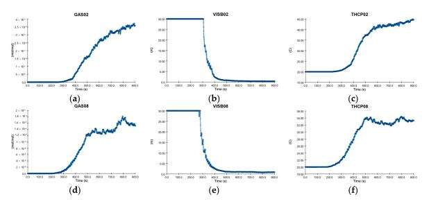
**Figure 14.** Change curves of fire characteristics under working condition A: (**a**–**c**): left transverse passageway; (**d**–**f**): right transverse passageway.
