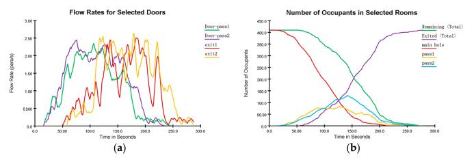
**Figure 17.** Results of evacuation simulation of working condition #1: (**a**) number of people passing through doors and exits; (**b**) relationship between the number of people and time in different areas.
