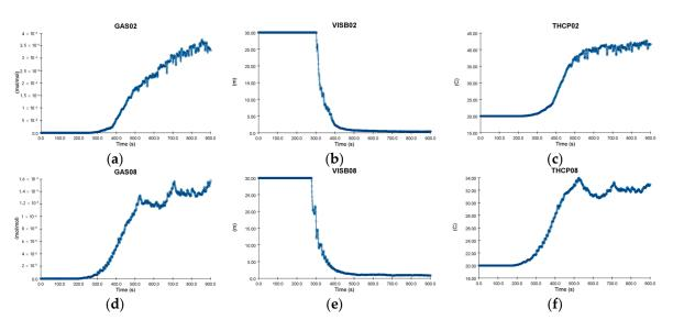
**Figure 15.** Change curves of fire characteristics under working condition B: (**a**–**c**): left transverse passageway; (**d**–**f**): right transverse passageway.
