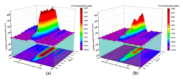
Figure 9. 3D curves of CO concentrations with time and distances: (a) 0.5 m/s; (b) 3.6 m/s.
