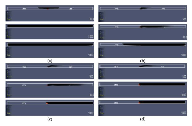
**Figure 4.** Front view of flue gas development with different longitudinal ventilation velocities. (a) 0.5 m/s, (b) 3.0 m/s, (c) 3.6 m/s, (d) 4.0 m/s.
