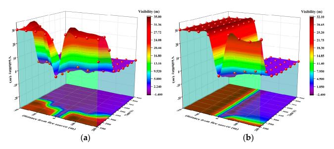
Figure 11. 3D curves of visibility with time and distance: (a) 0.5 m/s; (b) 3.6 m/s.
