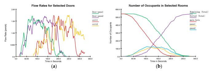
**Figure 18.** Results of evacuation simulation of working condition #2: (**a**) number of people passing through doors and exits; (**b**) time and number of people in different areas.
