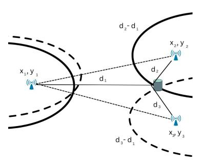
Figure 2. Localization based on Time Difference of Arrival (TDOA) measurement.
