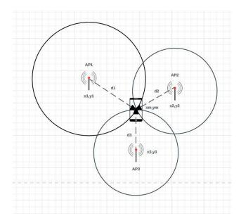
Figure 1. Localization Based on Time Of Arrival (TOA) Measurement.
