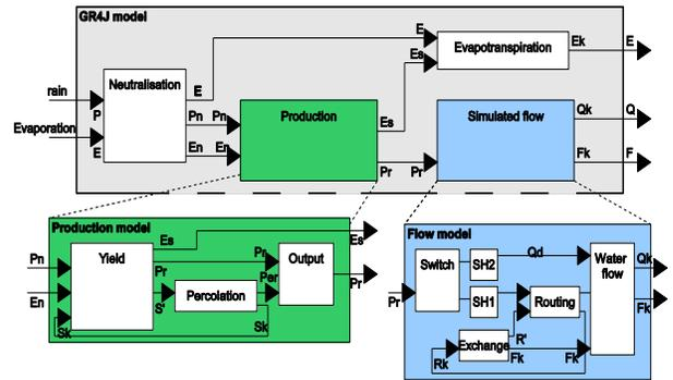
**Figure 2. Architecture of GR4J model**
