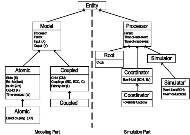
Figure 1. Correspondence between modelling and simulation in our approach
