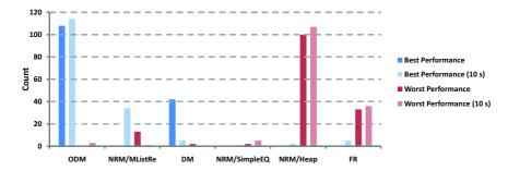
**Figure 9.4:** Best/worst performance counts for SSA algorithms. Blue bars denote the count of problems where the given algorithm outperformed all others, red bars denote the count of problems where the given algorithm performed worst. Counts from scenario three (using calibration) are dark blue and red, counts from scenario one (fixed simulation end time of 10 s) are light blue and red.
