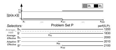
**Figure 2.2:** Average-effectiveness versus adaptive-effectiveness of a selection mapping. A list of sample selection mappings is ordered by their overall performance, with  $S^*$  being the optimal mapping.
