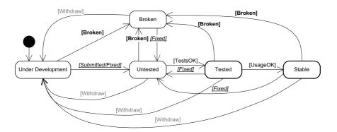
Figure 8.3: The plug-in life cycle considered by the AlgoSelectionRegistry, depicted as a UML state chart (e.g., [86, p. 121 et sqq.]). It is implemented in the class ComponentState. The colored transition guards of each kind all go to the same state: all fixed plug-ins are regarded as untested (underlined, italics), all plug-ins that fail are regarded as broken (bold), and all withdrawn plug-ins are regarded as being under development (gray).
