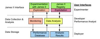
**Figure 4.6:** Overall architecture of the simulation algorithm selection framework. Two modules implement the interaction with the host system (Exploration and Exploitation, top layer), one implements data recording (Monitoring, middle layer), one the data analysis, and the two most general modules implement the storage of performance data and analysis results respectively (blue, bottom layer). Colors have the same semantics as in figure 4.5.
