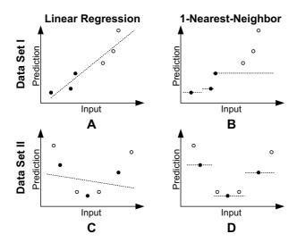
**Figure 2.4:** Prediction of linear regression (case A and C) and the one-nearest-neighbor approach (case B and D), compared on two data sets (cases A/B and C/D). Black dots denote sampled elements from which the prediction functions would have been constructed, whereas white dots show additional points of the underlying data distributions. The predictions of the two methods are sketched by dotted lines.
