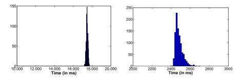
**Figure 2.11:** Two sample histograms of simulation algorithm runtime distributions in JAMES II. They are *not necessarily* heavy-tailed, as those considered in [114], but also not necessarily normally distributed either. Left: Execution times of 1000 flat-sequential PDEVS simulator runs on a  $100 \times 100$  FORESTFIRE benchmark model (see [134]). Right: Execution times of 1000 NRM-B simulator runs on a *CCS* benchmark model (see [158] or p. 231).
