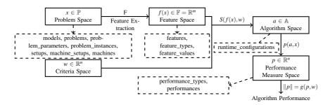
**Figure 5.2:** The algorithm selection problem as defined by Rice [272], and its mapping to concrete database entities (dashed boxes). The criteria space needs no representation within the database, as these preferences need to be given by the user (cf. fig. 2.3, p. 33).
