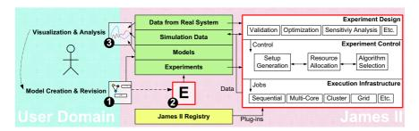
**Figure 7.2:** The experimentation layer of JAMES II (from [68]): After modeling (step 1), setting up simulation experiments (step 2) is necessary before any output can be analyzed (step 3). Arrows denote either data or control flow. While the experimentation layer (red box, right) comprises various components, the discussion here will be restricted to experiment design and control, i.e., some elements from the upper two layers of the red box.
