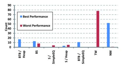
**Figure 10.4:** Best/worst performance counts for PDES algorithms. In contrast to the SSA case study (see fig. 9.4, p. 284), where only two algorithms dominated all others, here almost all algorithms outperform the others for at least one simulation problem (except for Time Warp and the sequential simulator using the simple event queue).
