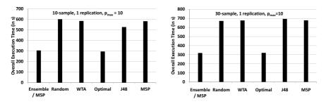
**Figure 8.8:** Impact of exploration sample size on selector performance. Sample size does not play an important role in this synthetic performance, as a linear relationship could even be derived from two samples only. While the ensemble selector (Ensemble / M5P) achieves near-optimal performance, neither decision trees nor model trees are able to clearly outperform random selection.
