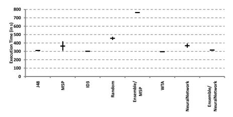
**Figure 9.10:** Real-world performance of selectors generated by different mechanisms, executed on nine formerly unseen CCS setups. Each experiment has been replicated ten times. Horizontal bars denote the average execution time, vertical bars display the standard deviation in both directions (i.e., average execution time  $\pm \sigma$ ).
