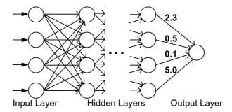
**Figure 6.9:** Basic outline of a neural network. Input is propagated from the input layer over the hidden layers to the output layer. Edge weights have been omitted for clarity, except for the single neuron of the output layer.
