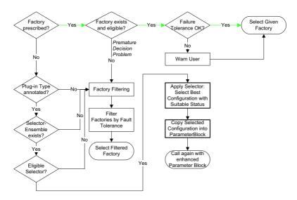
**Figure 8.7:** Flow chart of the selection procedure in AlgoSelectionRegistry. Bold borders mark the two actions that relate to automatic algorithm selection. Afterwards, getFactory(...) is called recursively, now with an augmented parameter block that prescribes which factory to be used. Ideally, subsequent calls to getFactory(...) follow the green arrows, i.e., the selected algorithms are able to cope with the given problem.
