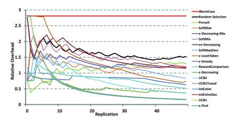
**Figure 10.5:** Relative overhead of policies on a PHOLD setup: the same plot as depicted in figure 9.6 (p. 290). Again, the legend on the right side is ordered by the policies' relative overhead after 50 replications. All policies are able to outperform a random selection, though their convergence speeds differ significantly. As before, worst-case and optimum performance have been estimated (see sec. 9.2.3, p. 289).
