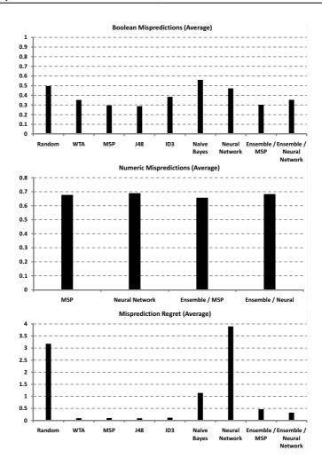
**Figure 10.7:** Selector performance estimated by the measures from section 6.2.2 (p. 193), similar to figure 9.9 (p. 297). Again, the numeric misprediction measure only applies to methods that give quantitative predictions. Misprediction regret (bottom) plots the performance overhead with respect to an optimal selection (i.e.,  $S^*$ ) in percent.
