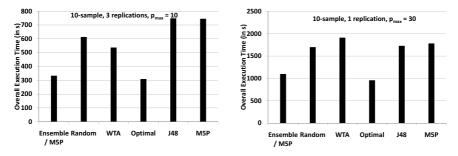
**Figure 8.9:** Impact of replication number and problem space size on selector performance. While the number of replications has little impact on selector performance, increasing the size of the problem space also increases the gap between the best selector (Ensemble / M5P) and the optimum.
