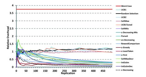
**Figure 9.6:** Relative overheads of the adaptive simulation runner, relying on the given policies to execute one of the six CCS setups. The legend on the right also reflects the final order of the policy overhead after 500 replications (top to bottom), i.e., UCB1 performs worse than random selection but the other policies perform better. The worst case scenario has been calculated afterwards, by considering the average performance of the worst algorithm.
