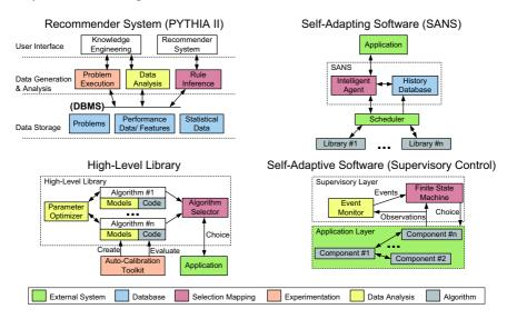
**Figure 4.5:** Software architectures for algorithm selection. Note that some components have several functions and are merely colored by their most important functionality, e.g., the intelligent agent component in the SANS layout (upper right) does *also* analyze the data stored in the history database. The sketches have been adapted from [146, p. 234], [60, p. 126], [176, p. 30–32], and [25, p. 81] (clock-wise, starting with upper left).
