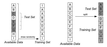
**Figure 6.10:** Bootstrapping: instances are drawn randomly, the rest is used as test set.
