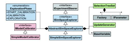
**Figure 7.17:** The main components for simulation space exploration in JAMES II: the simulation space explorer (blue), the calibrator (red), and the parameter block management (green). Most are linked with fundamental JAMES II entities (grey). Plug-in types are marked by bold dotted borders.
