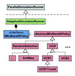
**Figure 7.8:** UML class diagram of the adaptive simulation runner and auxiliary components (from [72]): existing components (grey), the simulation runner implementation (green), the policy interface (blue), and the policy implementations (red). JAMES II plug-ins are denoted by dashed borders.
