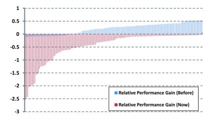
**Figure 9.5:** Relative performance gains before and after the code change. Note that, for the sake of clarity, the performance gains are sorted independent of each other in ascending order, so two bars at the same position do *not* represent the same problem.
