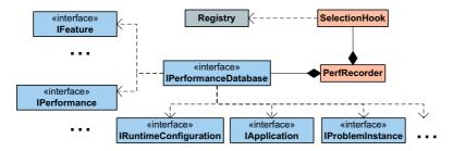
**Figure 5.5:** UML diagram of the most relevant components for data recording and storage in the SASF. For full flexibility, all concrete implementations of performance data entities are hidden by interface definitions. The colors again denote different parts of the SASF: data storage (blue) and monitoring elements (orange), see figure 4.6 (p. 148).
