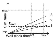
**Figure 7.16:** Calibration means to identify a simulation end time so that algorithms of differing speed (1: slowest, 3: fastest) finish execution after  $\approx t_{opt}^{wct}$  wall clock time. The quasi-steady state property of the model is presumed, so the relationship between wall-clock time and simulation end time is *linear*.
