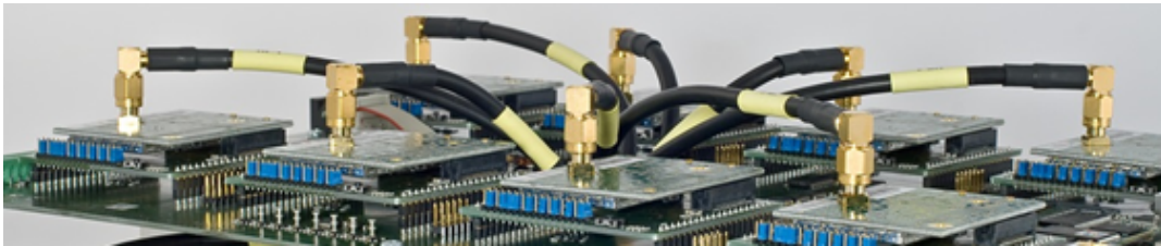
Figure 3.4: RoSeNet radio emulation and test platform hardware panel (taken from [55])
