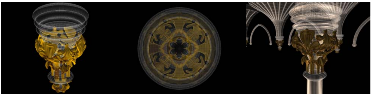
Figure 1: Print renderings utilizing wireframe to show distinction between carved and milled moldings on column capital.
