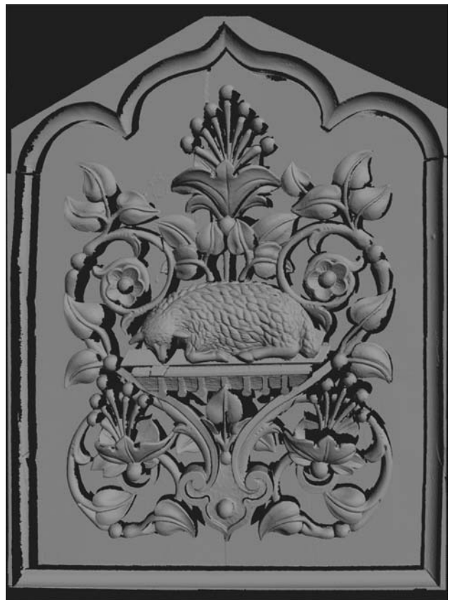
Figure 3: A close-range laser scan of altar detail via a ShapeGrabber PLM600 provides a level of detail accurate enough to create realistic reproductions.
