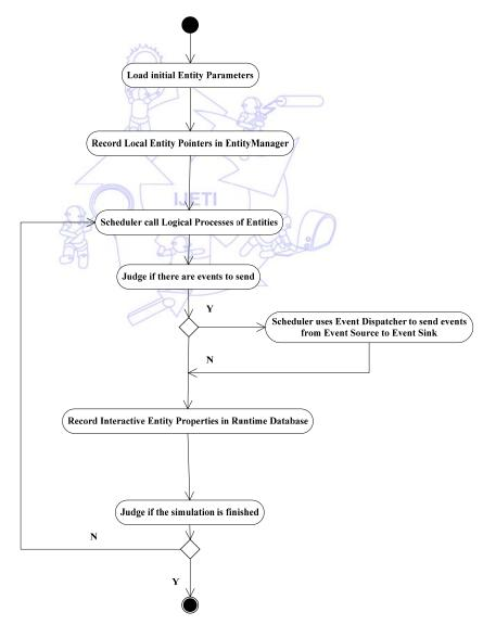
Fig. 3 Running Process of Simulation Engine
