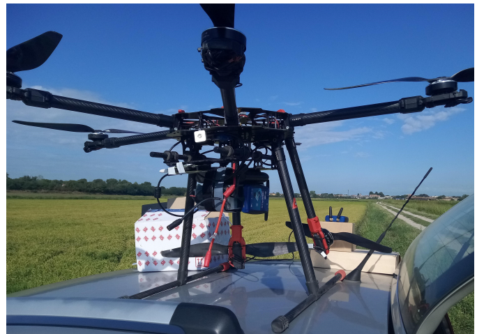
Fig. 10: The Tarot UAV in its complete configuration: the ADALM Pluto SDR as RF front end and the Raspberry Pi with the SenseHat IMU board for data logging.
