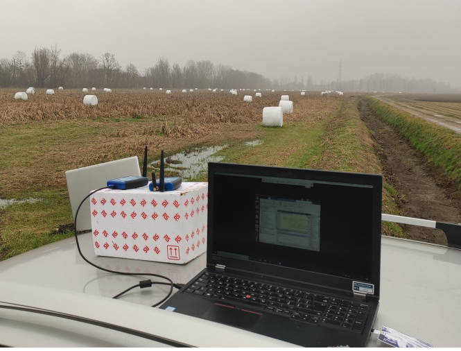
Fig. 1: Experimental setup of the ground-to-air link. There are two ADALM-Pluto SDRs on the roof of a car: one is the transmitter and the other is used for monitoring.
