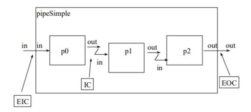
Fig.6 Coupling in a DEVS coupled model
