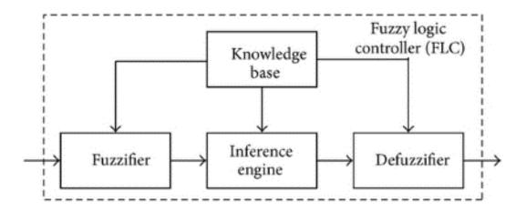
Fig.9 Simple architecture of a FLC
