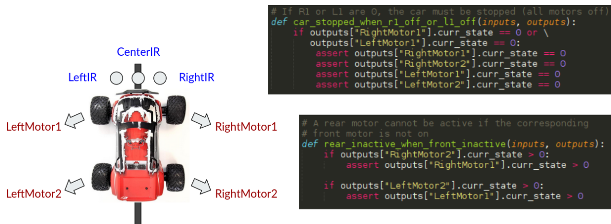
Figure 3.14: Sample example of metamorphic rules definition through Python functions.
