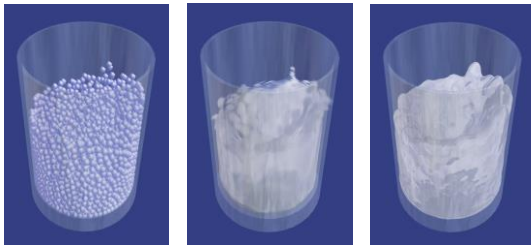
FIGURE 10. A swirl in a glass induced by a rotational force field. (a) Particles, (b) surface using point splatting and (c) iso-surface triangulated via marching cubes. [99]
