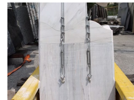
Figure 7. Steel wires on Fallacara's arch [18].
