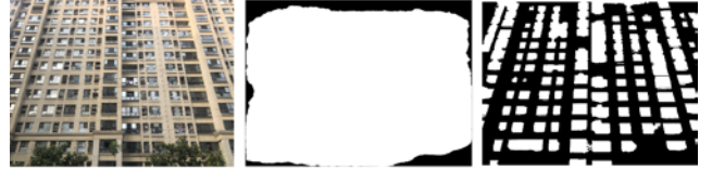
Figure 2. A building elevation image and the wall and windows recognized by the AI
