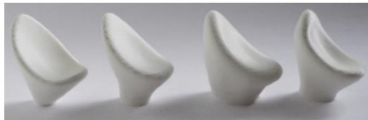
Figure 18. 3D printed models. From right to left: Input shape, GD, LSM and Solver modified shapes.
