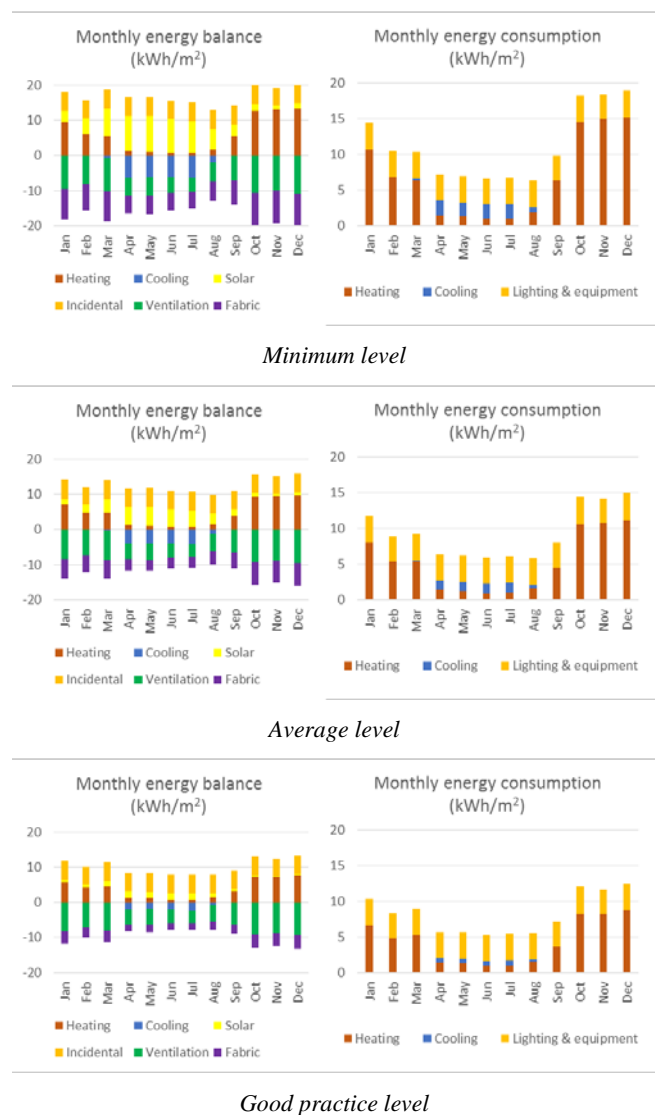
Figure 6. Comparison of the impact of three levels of building fabric design on annual energy consumption (kWh/m 2 /year)
