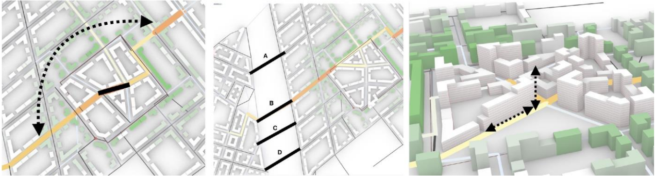
Figure 5. Parameter of the generative model. From left to right: Angle of central street segment, bridge location, building volumes.
