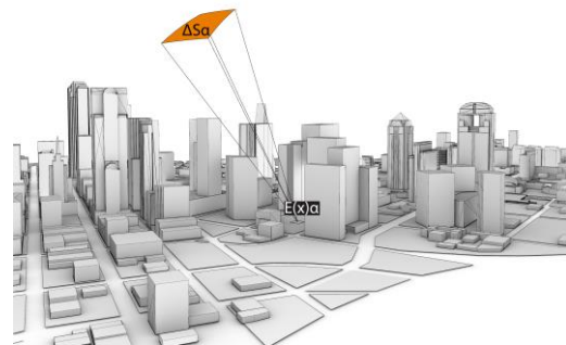
Figure 5. Radiation from a single sky patch being measured in an urban context.
