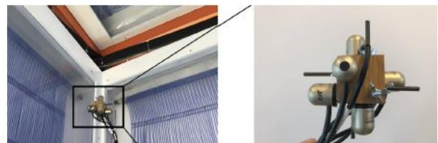
Figure 9. Pyrgometers arranged orthogonally on a wooden cube inside the pavilion at the location shown in Figure 8.
