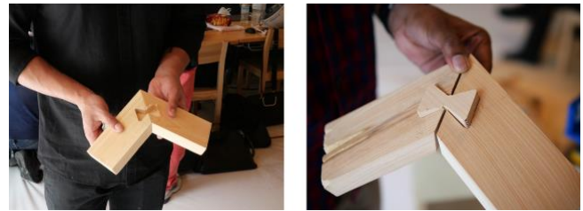
Figure 10. Tolerances drastically increased during fabrication of complex joints.
