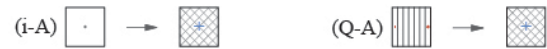
Figure 5. Absorber panel rules replace either an initial shape or an N7 QRD panel with a shape representation of an absorber panel.
