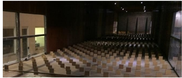
Figure 7: Wind tunnel interior: roughness blocks and spires.
