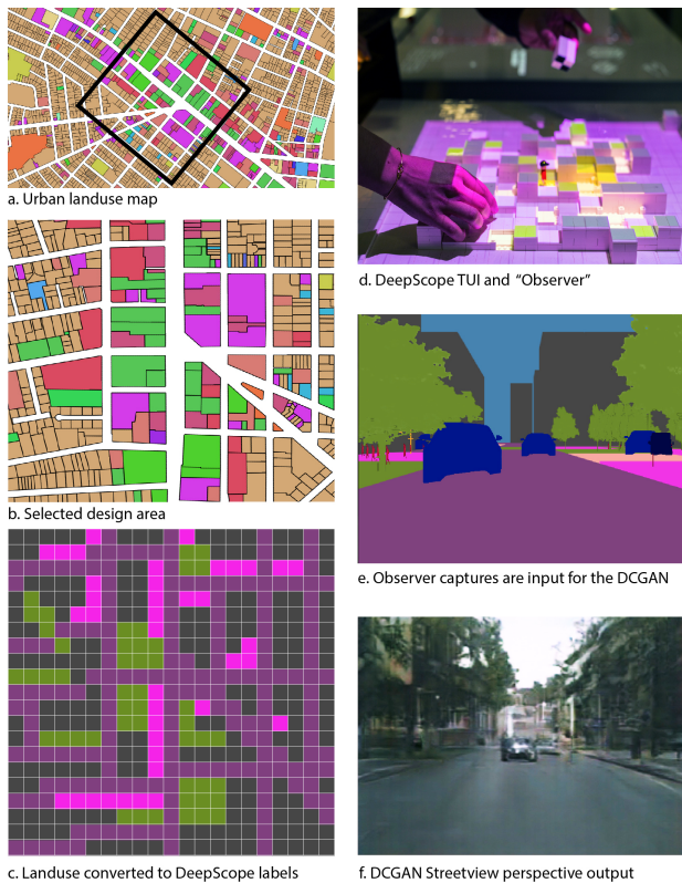
Figure 3. DeepScope process: (a,b) designating an urban intervention site (c) translating the site's land-use/zoning bounds and (d) user-interaction into (e) procedural 3D environment and (f) passing it to DCGAN model for generation of a street-view visualization
