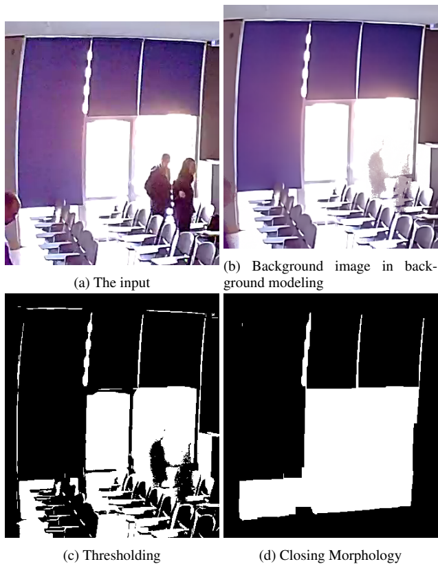
Figure 3: The steps of the curtain openness ratio estimation
