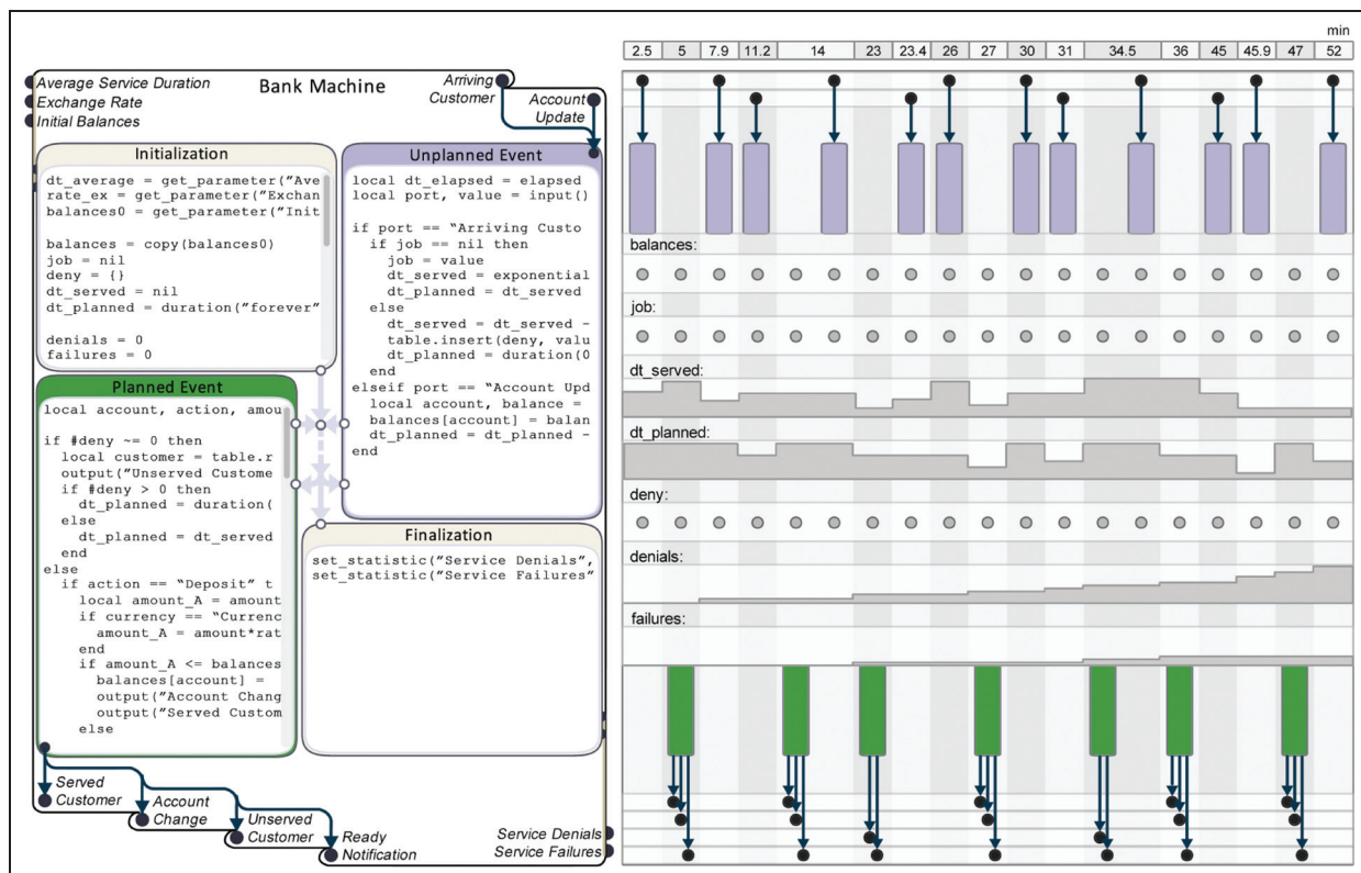
Figure 2. The atomic class debugging tool, consisting of the code view and the visualization of events with messages and state variables displayed in the timeline on demand.
