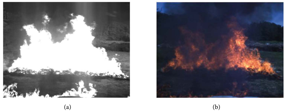
Figure 3. Images of a fire producing dense black smoke in the visible spectrum (a) and in the near infrared spectrum (b).
