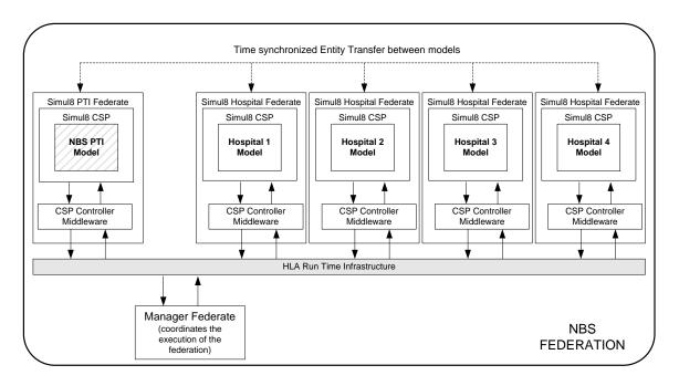
Figure 5: The NBS Distributed Simulation Federation comprising of one NBS-PTI model, four NBS-Hospital models and one Manager Federate. The CSP Controller Middleware is the interface between the CSP Simul8™ and HLA RTI.
