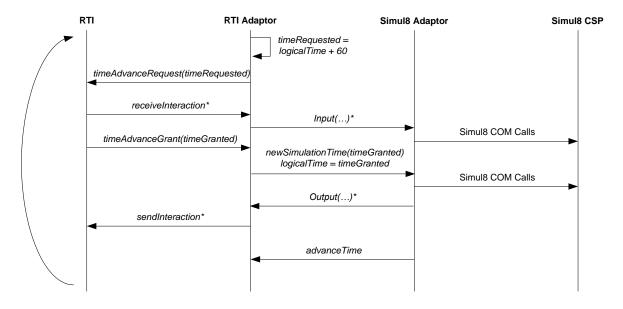
Figure 6: CCM communication protocol showing the interactions between a federate (e.g., NBS PTI centre, hospitals, manager federate) and the HLA-RTI
