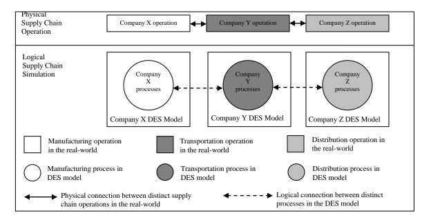
Figure 1: Modern supply chain with organisations X, Y and Z involved in manufacturing, transportation and distribution operations respectively. The logical simulation processes representing these operations are contained in three different DES simulations, each representative of the physical operation associated with a specific organisation.
