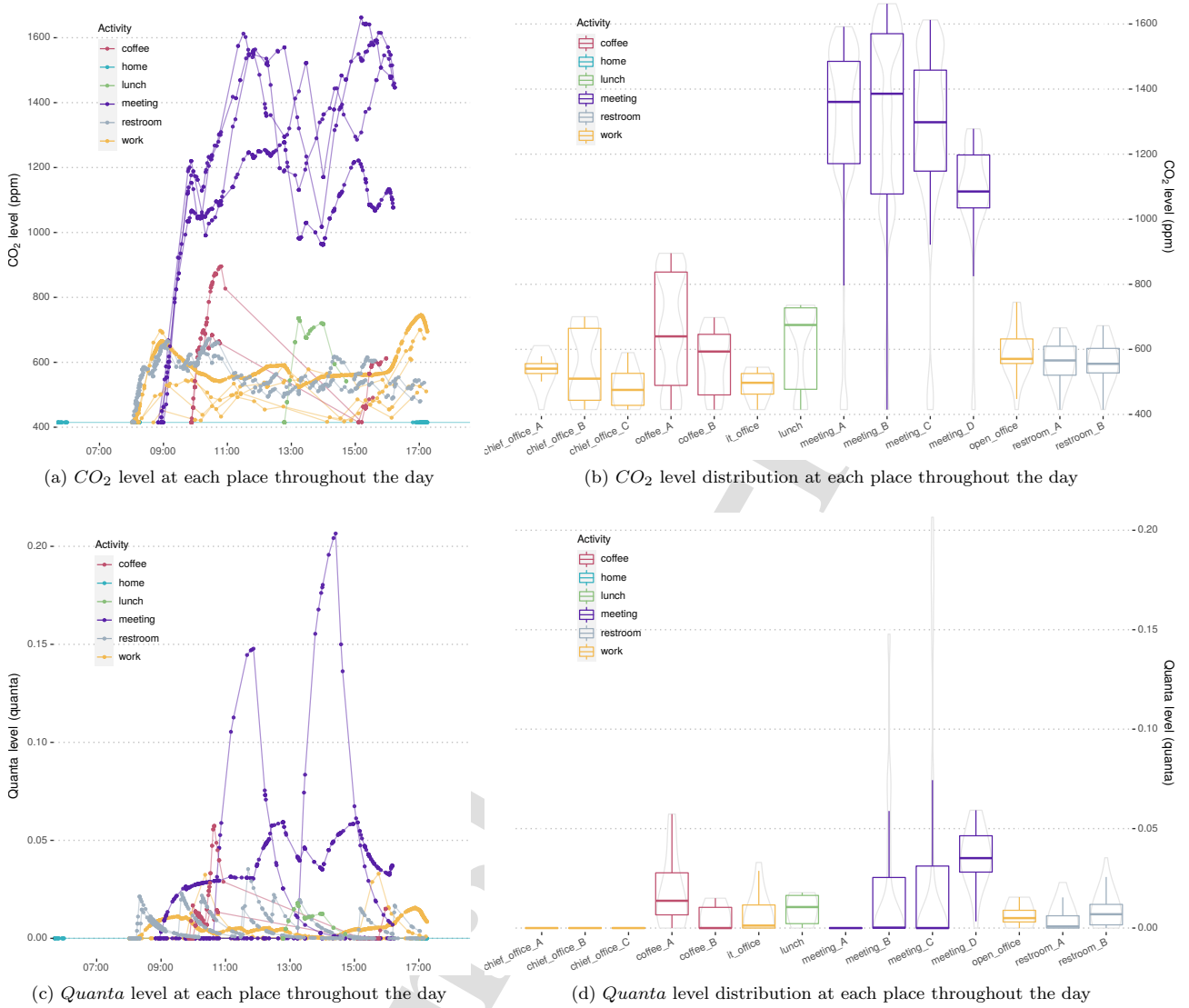
Figure 9: Baseline experiment results: indoor air quality at place-level with CO_2 and quanta levels
