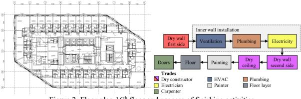
Figure 2: Floor plan 16th floor and process of finishing activities
