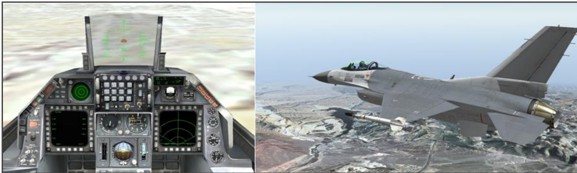
Figure 10: SIMbox training environment for an F16 fighter. This environment can be integrated with an actual cockpit (with joysticks, etc.) to provide more realism.
