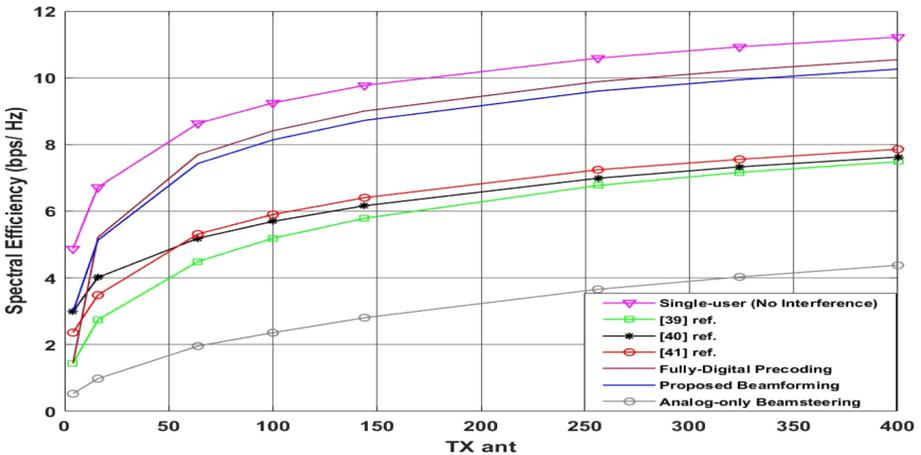
Fig. 6. Spectral efficiency against the BS antennas
