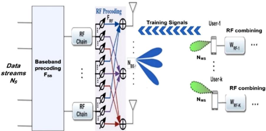
Fig. 2. The proposed hybrid beamforming for femto-cells.
