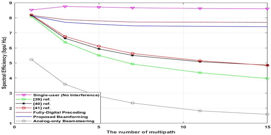
Fig. 7. Spectral efficiency against the number of multi-path.
