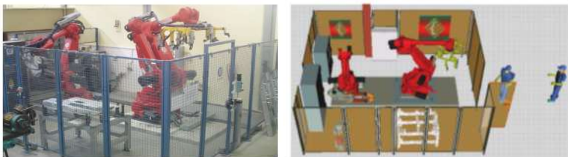
Figure 7. Real assembly cell (left) vs virtual assembly cell (left) (Makris, et al., 2012)
