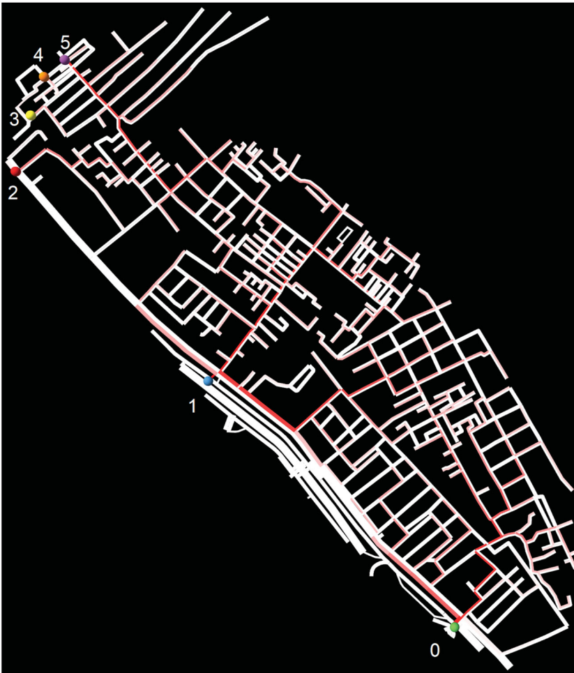
Figure 12. Road network displaying the shortest path between a building, and its closest evacuation point. The width of the road is proportional to its number of lanes. The spheres represent the evacuation points. The color of roads depends on the number of times they have been part of a shortest path to an exit point: the more it is red, the more it supposed to be used by the agents to evacuate the area.
