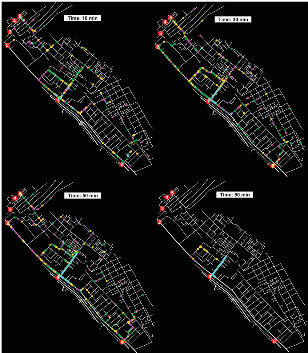
Figure 5. Example of a mixed traffic simulation results at different time step. In cyan, cars; in magenta, motorcycle; in yellow, bicycle; in green pedestrian. This example shows the main traffic jam area near exit number 1.
