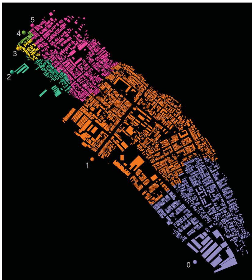
Figure 2. Sectorization of buildings according to the nearest evacuation point using the road network. The spheres represent the exit points, the color associates a building with the nearest exit.
