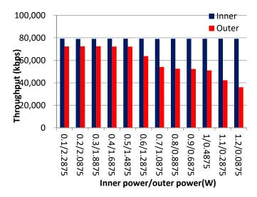
Figure 4. Power allocation VS. inner/outer area throughput.
