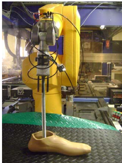
Figure 1. Robot test cell with a simple foot prototype
