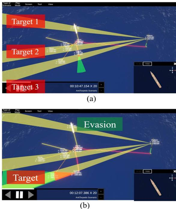
FIGURE 12. DVES screenshots of surface ship evasive maneuvers. (a) Submarine target detection. (b) Surface ship evasive maneuvers.
