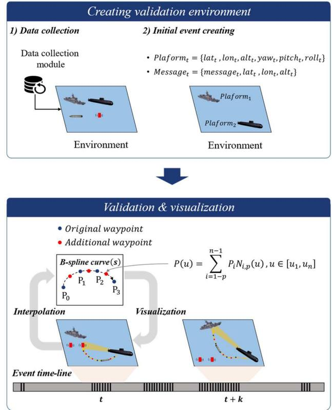
FIGURE 5. Brief description of the scenario for maneuver validation of a submarine.
