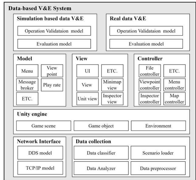
FIGURE 8. Architecture for DVES implementation.
