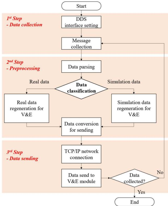
FIGURE 4. Operational flowchart of the data collection module.
