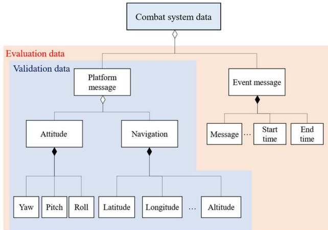
FIGURE 7. Message modeling diagram for combat system engineering.
