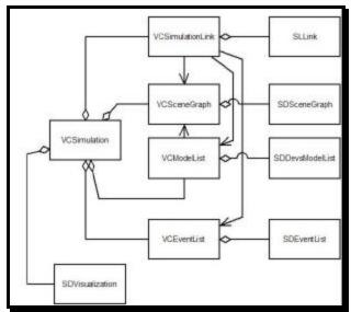
Figure 10: ViewerControl and SimulationDatabase.
