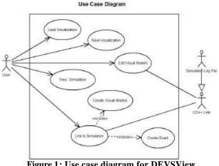
Figure 1: Use case diagram for DEVSView
