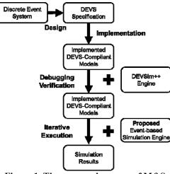
Figure 1. The proposed process of M&S
