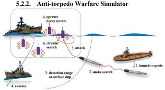
Figure 8. Brief scenario of anti-torpedo simulation [3]
