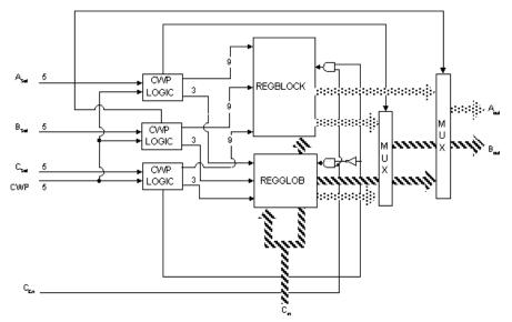
Figure 10. Architecture of the processor's registers.
