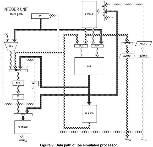
Figure 9. Data path of the simulated processor.
