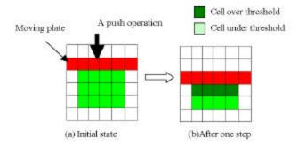
Fig. 3. Push operation by a moving plate.
