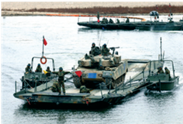
Figure 1. Ribbon Bridge System (raft) 7 .
