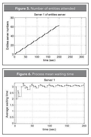
system will supply. The server's behavior, according to the serviced units is linear in function of time, ensuring a smooth transition in this workstation, including that at certain times the workstation remains idle, with no products to deliver to the next workstation.
