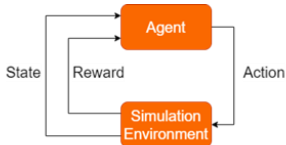
Figure 2.1 - Agent-Environment interaction diagram, adapted from [17]
