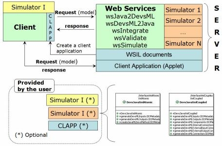
Figure 7: Web service Architecture for DEVSML Implementation
