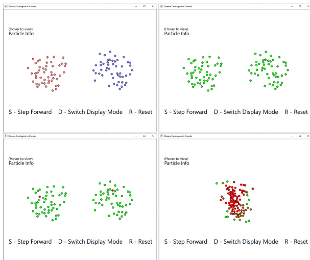
Figure 11: Snapshot from our interactive framework for simulating disease spreading in moving crowds. Typing “D” switches the display mode between showing particle groups (top left) or particle disease status (top right), while clicking any particle can mark that particle as fully infected, turning its color to red ( \beta = 1 , see bottom left). Typing “S” advances the simulation by ten time steps, showing the details of the disease spread (bottom right).
