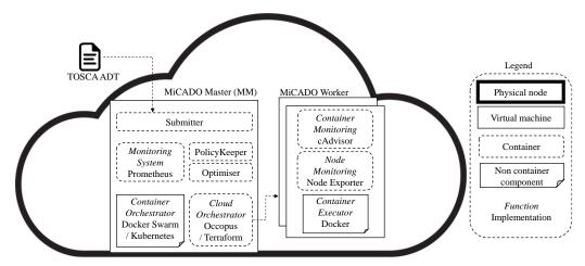
Figure 6: High-level architecture of the MiCADO cloud orchestration framework.
