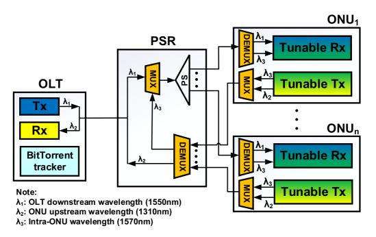
Figure 1. Proposed BitTorrent locality-aware process in the EPON system architecture
