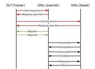
Figure 3. BT operation in the EPON
