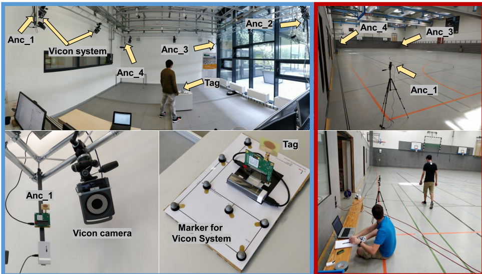
Figure 4.11: Set-up for the experimental evaluations conducted at the laboratory environment in CITrack [119] and University's indoor sport hall arena.
