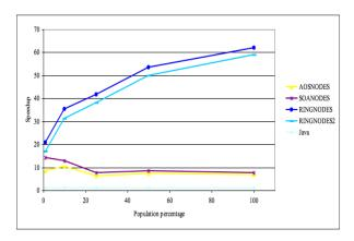
Figure 7. GTX 280 Speedup Relative To Java Implementation
