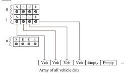
Figure 5. Administration Structure Implemented As A Ring Buffer
