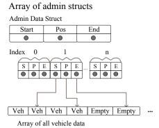
Figure 2. Administration Structure For Vehicle Data On Link/In Buffer
