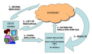
Figure 6: Execution of DEVS SOA-Based M&S
