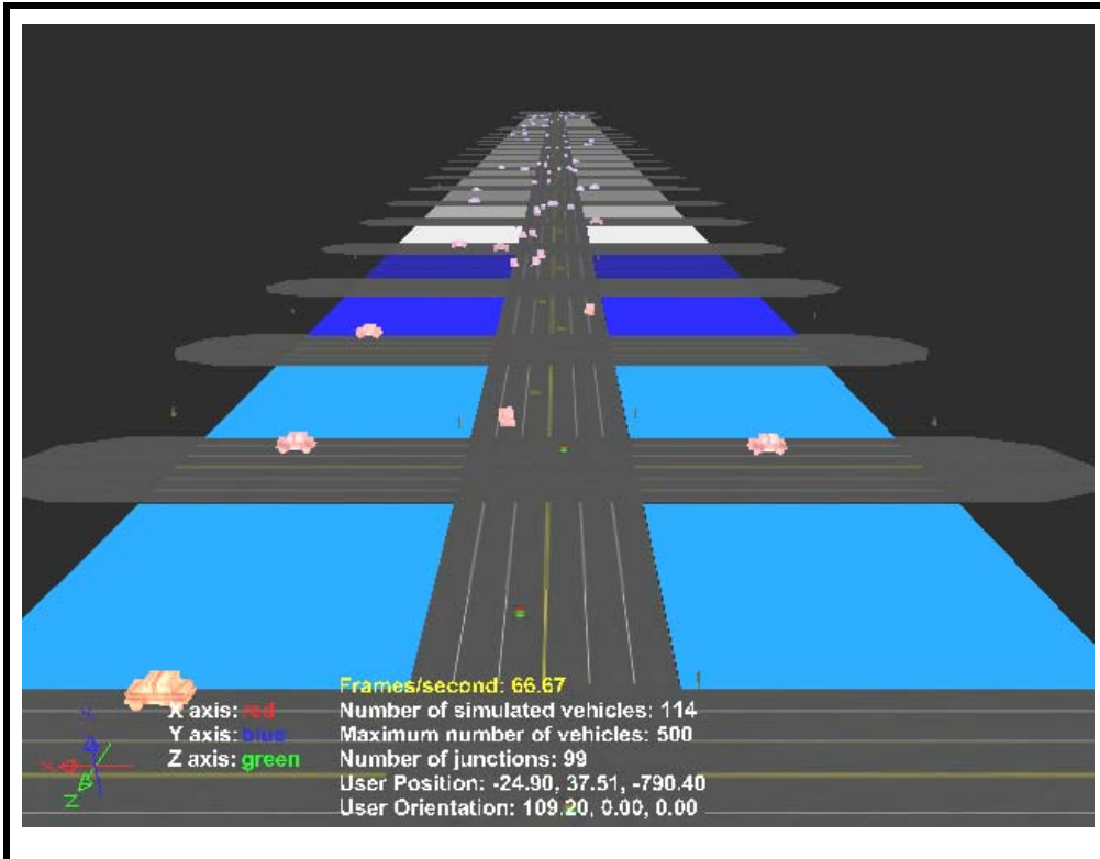
Figure 24: Visualization of terrain and vehicle LODs for an automatically generated traffic graph.
