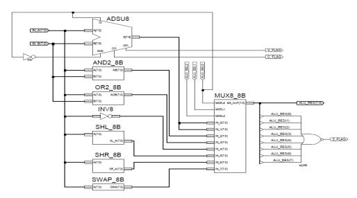
Fig. 7. Arithmetic and Logical Unit schematic diagram
