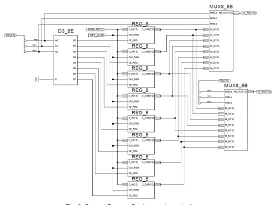
Fig. 6. General Purpose Registers schematic diagram
