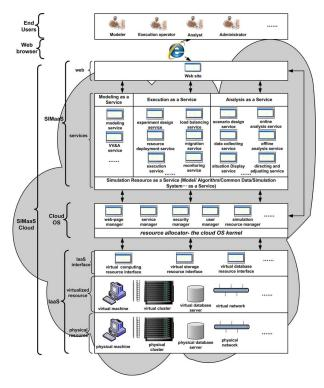
Fig. 3. The architecture of the Cloud Simulation [44]
