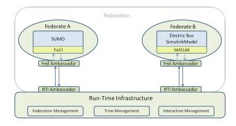
Fig. 2. HLA's Functional Architecture with two different simulators [23]
