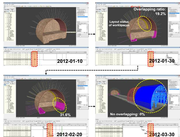
Fig.8. 4D Simulation of the Workspace Overlapping Status
