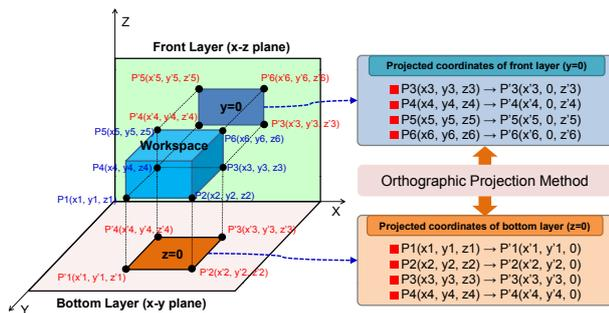
Fig.3. Orthographic Projection Method of the Bottom and Front Faces for Workspace Models
