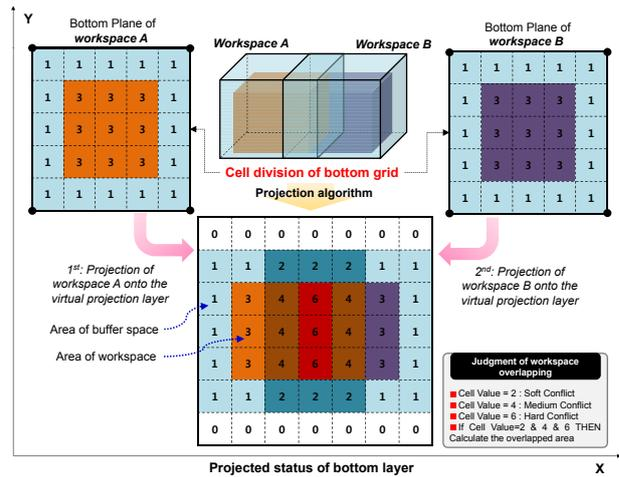
Fig.4. Overlapping Cell Calculation and its Judgment between the Workspaces A and B Projected onto the Virtual Projection Grid Layer
