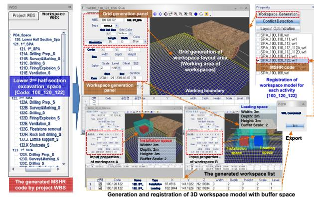
Fig.6. Generation and Registration of a 3D Workspace Model for the Activity
