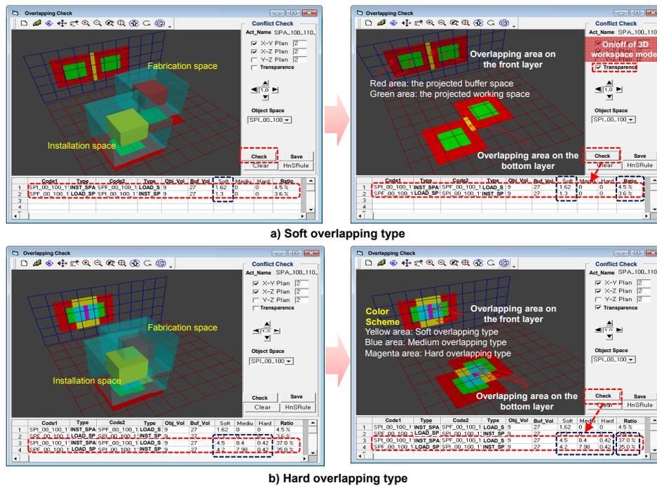
Fig.7. Overlapping Visualization of Two Workspaces and its Overlapping Type
