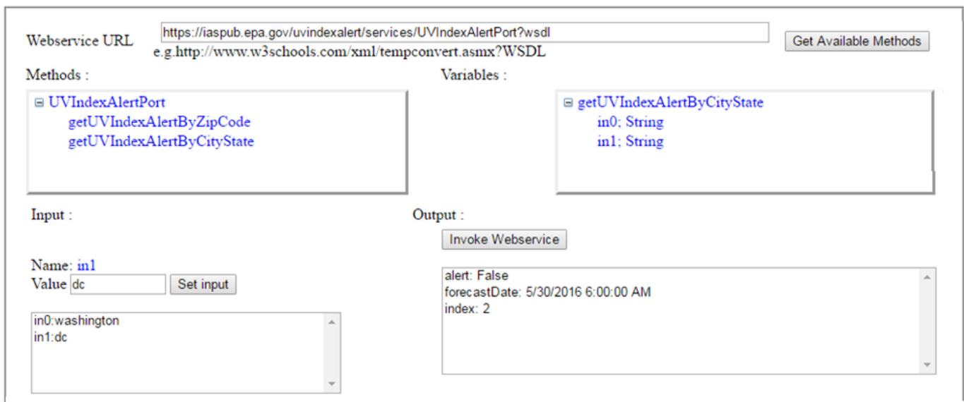
Fig. 5. User interface for runtime access of web service based models, the case of EPA's UV alert web service.
