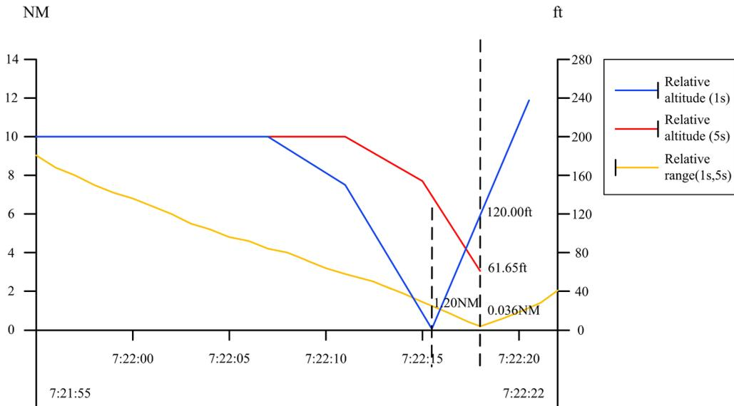
Fig. 9. Relative range and altitude between Aircraft 1 and Aircraft 4 with the pilot response time of 1 s and 5 s.
