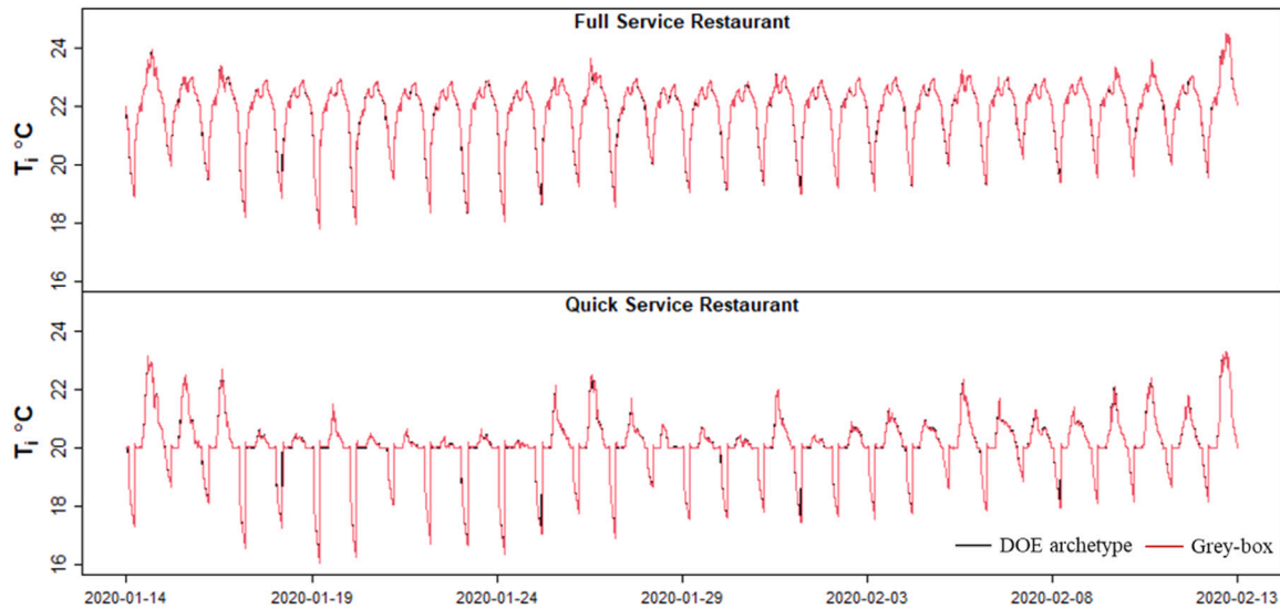
Fig. B.3. Higher order model DOE archetype and grey-box internal temperature profiles for the full service and quick service restaurant DOE archetypes at the whole building level over a four week period.
