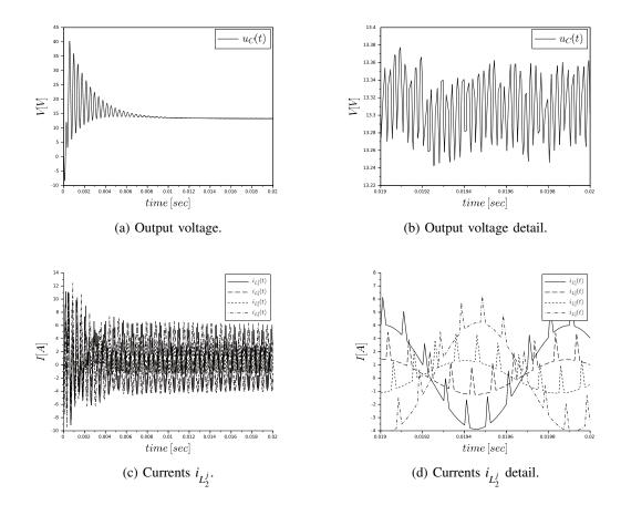
Figure 2: Four-stage Ćuk converter simulation results.
