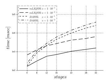
Figure 3: Four-stage Ćuk interleaved converter simulation time comparison.
